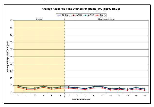
IOPS Test Run - Response Time Frequency Distribution Data
