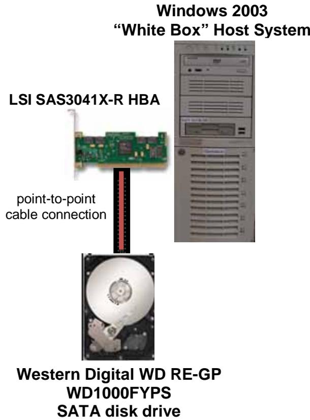
**Benchmark Configuration/Tested Storage Configuration Components**
