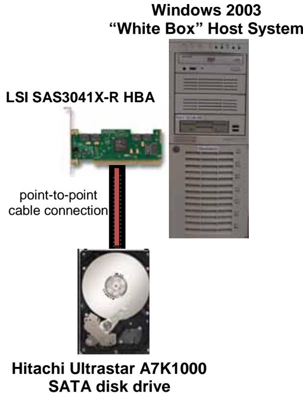
**Benchmark Configuration/Tested Storage Configuration Components**
