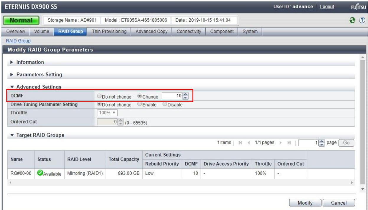
The screenshot displays the Fujitsu ETERNUS DX900 S5 management interface. The user is logged in as 'advance'. The 'RAID Group' tab is selected, and the 'Modify RAID Group Parameters' window is open. The 'Advanced Settings' section is expanded, and the 'DCMF' parameter is set to 10, which is highlighted with a red box. The 'Target RAID Groups' table shows one RAID group (RG#00-00) with a DCMF value of 10.
